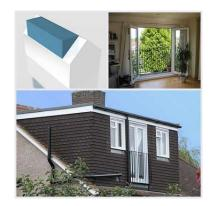
The Dormer is a structure projecting from the roof slope, which lets in additional light and ventilation to the loft conversion. A dormer will also enable additional headroom.
